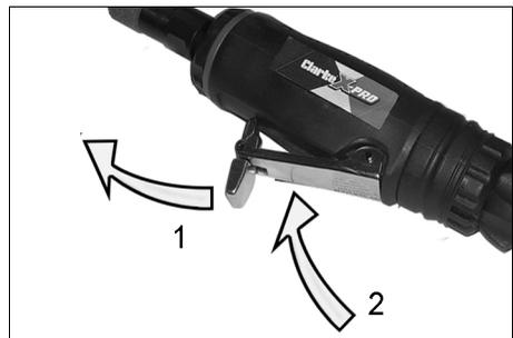
3. Release the trigger to stop the grinder.
